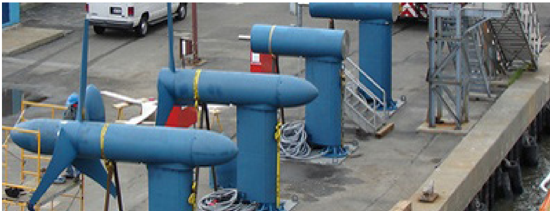
35 kW units shown before deployment in the East River, New York, United States.
